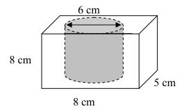
A hole 6 cm in diameter is bored through a square nut made of copper. If the square nut is 8 cm to a side and 5 cm thick, find the total volume of copper used to make the nut after the hole is cut.
